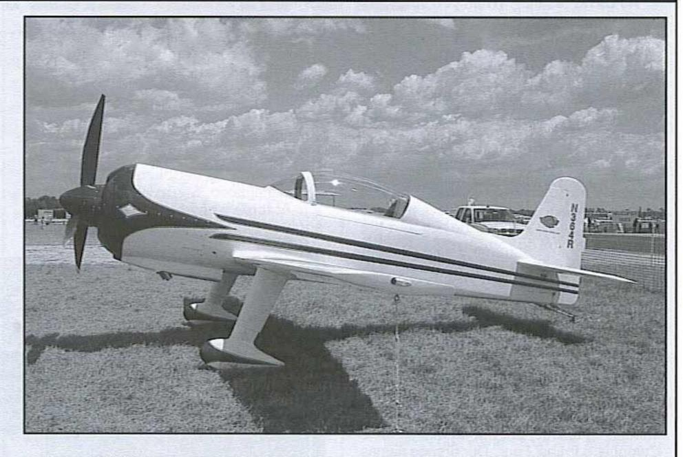
and over 2,000 fpm at gross. Stall with the flaps down occurs at 68 mph. Vne is 280 mph. G limits are +6, -4 (limit) and +9, -6 (ultimate). The empty weight is 1,650 lbs. and gross is 2,450.
